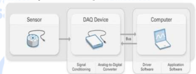
Gambar 2. Diagram blok bagian sistem Data Acquisition
