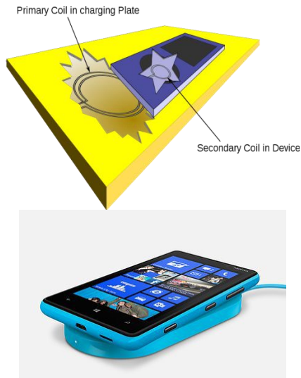
Figure 3. Wireless charging Workflow
