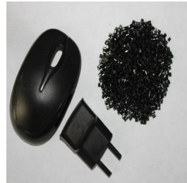
Figure 4. Polycarbonate/Acrylonitrile Butadiene Styrene (PC/ABS) plastic
