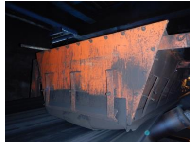
Figure 10. Tailbox extension at transfer point area
