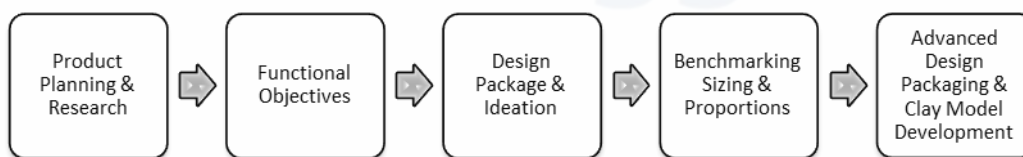
Gambar 2. Advanced Concept Design Process (Stuart Macey, 2009)
