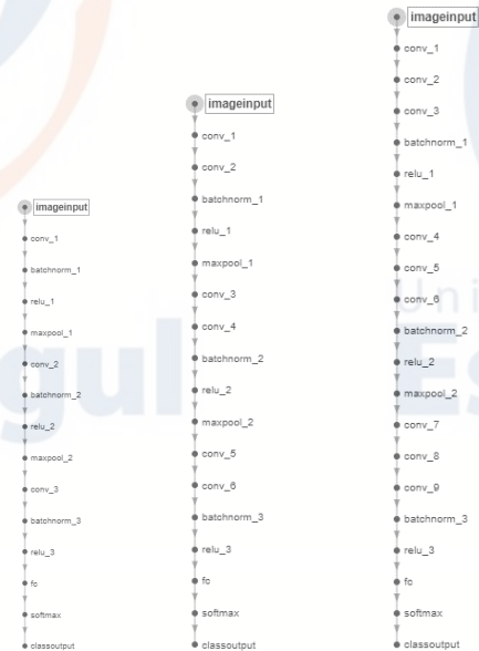
Fig. 3 The architecture of the 3 AlexNet models based on the variation in the number of convolutional layers in each block (left) AlexNet 1 (middle) AlexNet 2 (right) AlexNet 3.
