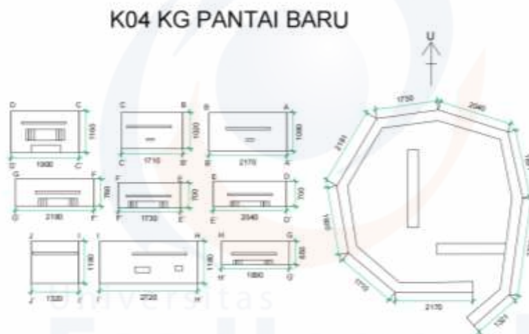
Figure 16: Measurements of the British pillbox at Kg Pantai Baru, Bachok, Kelantan. Source: Field study.
