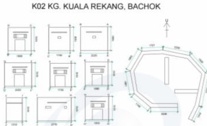
Figure 11: Measurements of the British pillbox at Kg Kuala Rejang, Bachok, Kelantan. Source: Field study.
