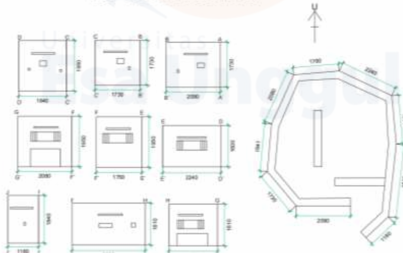
Figure 20: Measurements of the British pillbox at Kg Pantai Chap, Bachok, Kelantan. Source: Field study.
