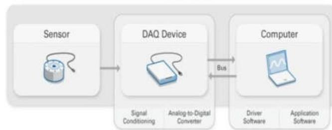
**Gambar 4. Diagram Blok Sistem Data Acquisition (Alfanz et al, 2016)**
