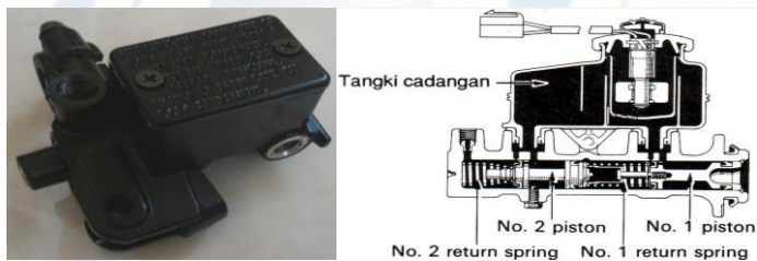
Gambar 2.1 Master cylinder
