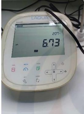
A digital pH meter with a white casing and a black LCD screen. The screen displays a pH value of 6.73 and a temperature of 20.7°C. The meter is connected to a glass electrode probe.  | <p>Hasil pengujian pH hari ke-2 (6,73)</p> |
