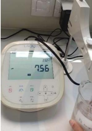
A digital pH meter similar to the one in the first row. The screen displays a pH value of 7.56 and a temperature of 23.2°C. A hand is visible holding a glass beaker next to the meter.          | <p>Hasil pengujian pH hari ke-6 (7,56)</p>  |
