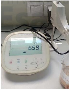
A digital pH meter with a white casing and a black LCD screen. The screen displays a pH value of 6.59 and a temperature of 20.7°C. The meter is connected to a glass electrode probe.   | <p>Hasil pengujian pH hari ke-1 (6,59)</p> |
