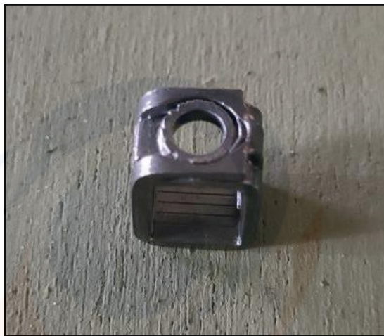
Gambar 1. 1 Terminal Clamp M5 (Semi-finished product) (Sumber : Pengamatan di PT. Anugerah Sinbet Mandiri)
