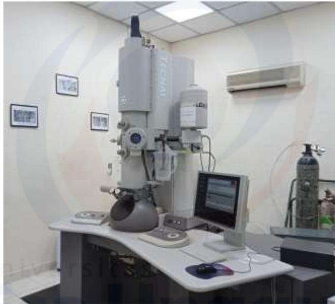
Gambar 10. ALat **Transmission Electron Microscopy (TEM)**
